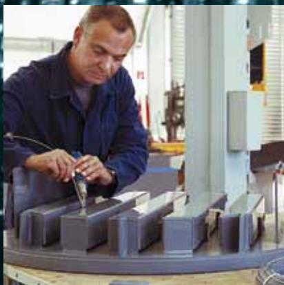
Fabrication of a thermoplastic tray
