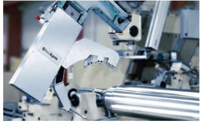
HCC KPM integrated 4-probe measuring caliper for 3D measuring and dynamic on-line shape correction capabilities
