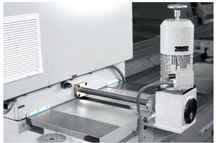
Motor and drive spindle for X-axis movement
