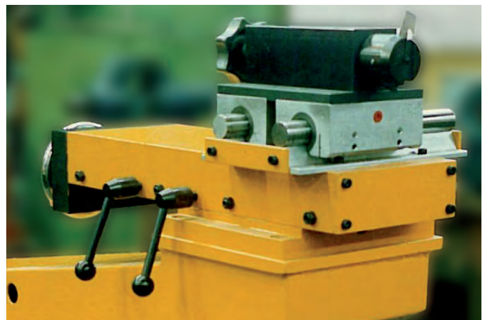
System installed on a floating supporter to follow the groove-inclination for cleaning the grooves respectively the groove edges
