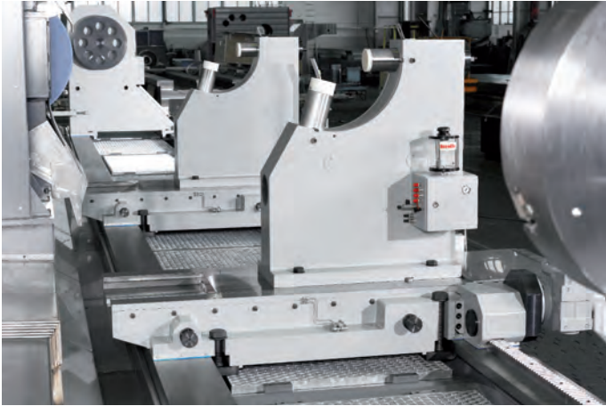
Steadies on lower parts for centerline displacement of steadies (in the rear, calibration disk at tailstock)
